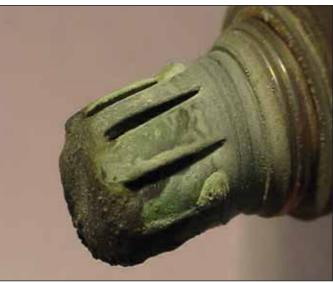
This oxygen sensor has been contaminated by engine coolant and silicone. Its output skewed low, giving a false lean indication to the PCM.
