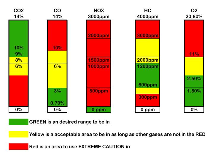
The bar chart above shows acceptable exhaust gas ranges during Idle Tuning for CO2, CO,NOX, HC and O2. These are general that would apply to most engines and base line readings
