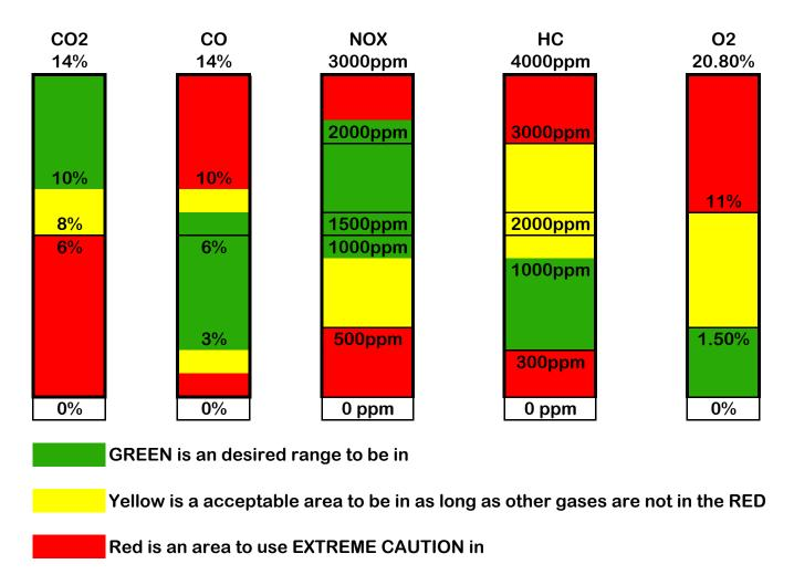
The bar chart above shows acceptable exhaust gas ranges during Peak HP for CO2, CO,NOX, HC and O2. These are general that would apply to most engines and base line readings
