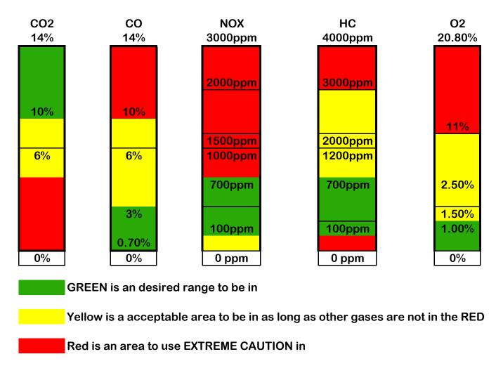
The bar chart above shows acceptable exhaust gas ranges during Idle to Steady State for CO2, CO,NOX, HC and O2. These are general that would apply to most engines and base line readings
